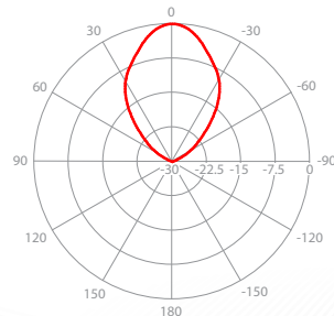
V/H - Port Pattern Elevation 5.6 GHz
